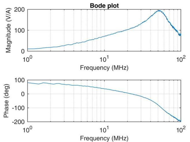
Fig. 7. Bode diagram of the magnetic loop antenna.
