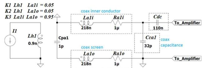
Fig. 3. Equivalent electric circuit of the magnetic antenna.
