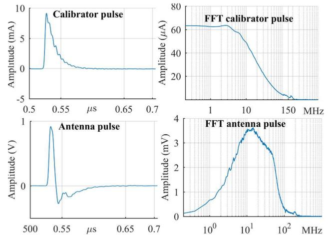
Fig. 6. Magnetic antenna response to a calibrator pulse.
