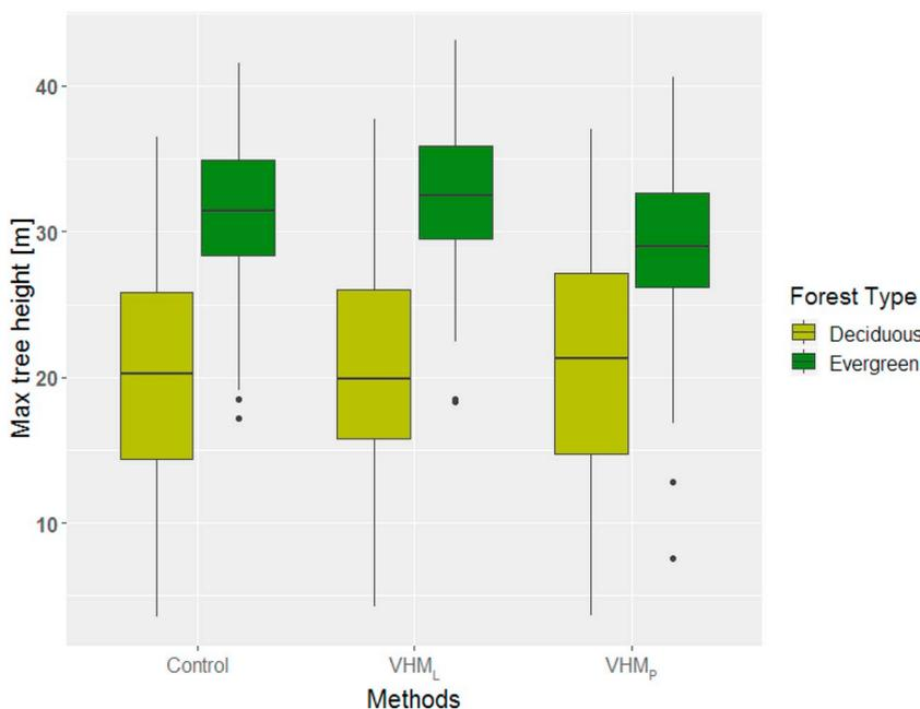
Fig. 3. Tree height measured with different methods (in the field using Vertex as control method, and derived from the models based on LiDAR and photogrammetric DSM). The  $VHM_L$  provides estimates with smallest differences to control method in both forest types (deciduous and evergreen) and overestimates the heights. The  $VHM_p$  overestimates heights in the deciduous forest type and underestimates heights in the evergreen forest type.
