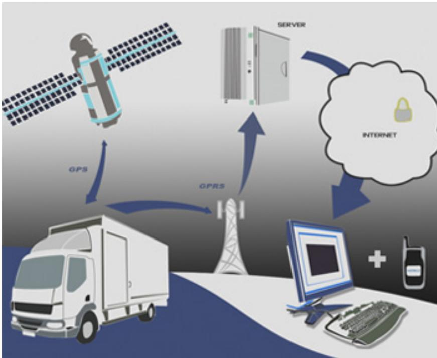
**Figure 3. Vehicle tracking system.**
