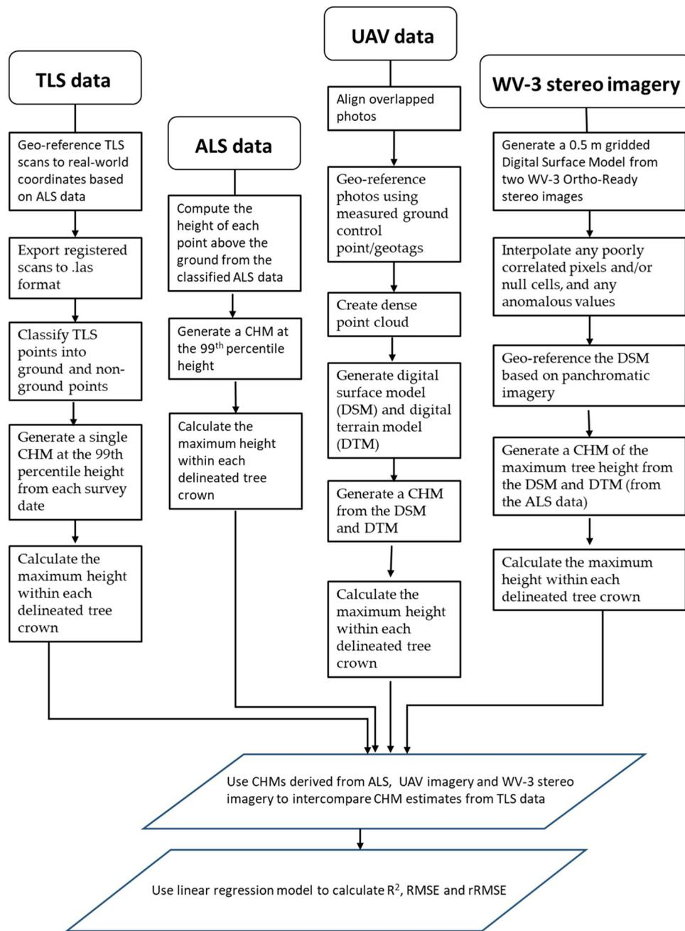
Fig. 2. Flowchart of evaluating the accuracies of canopy height estimates from Ground Laser Scanning (TLS) data, Airborne Laser Scanning (ALS) data, Unmanned Aerial Vehicle (UAV) imagery and WorldView-3 (WV-3) stereo imagery.
