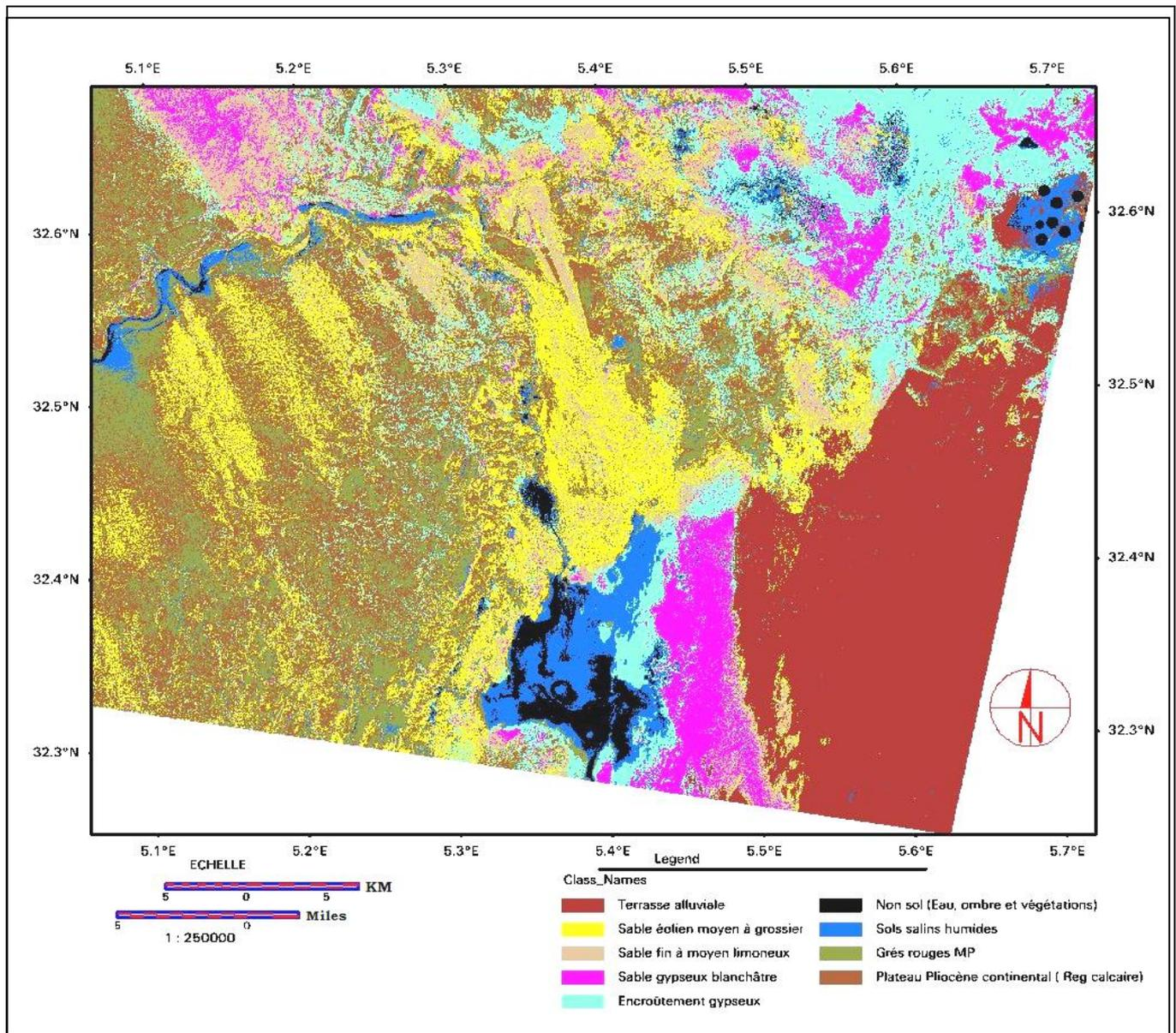
encrusting surface formation; 6 - surface formation: wet saline soils and saline efflorescence (Hamdi-Aissa, B. 2004) [5]; 7- continental Pliocene plateau surface formation (Reg limestone); 8- Surface red sandstone Mio-Pliocene.
